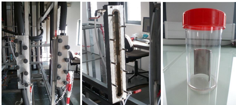
Figure 2: Alphéo II, view of sampling boxes and stainless steel coupons
